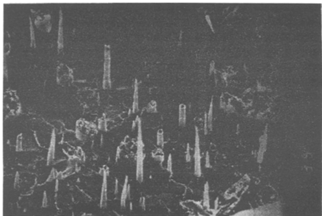
Fig. 11. Morphology of blend extrudate at 10% content of LC component (white fibers).
